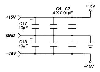
C4 - C7 connect as closely as possible to the power pins of IC2 and IC3.
